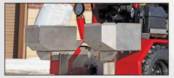
**MATERIAL HOLDING TRAYS** Additional gear, fuel and deicing materials are in easy reach when material holding trays are added, saving time and money on the job by helping operators beat the clock.
