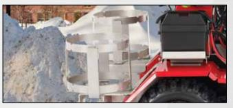
**5-GALLON BUCKET MOUNTS** Optional 5-gallon bucket mounts attach quickly and simply to Snowrator® and give an operator easy access to additional deicing materials on the back of the unit.
