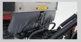
An exclusive salt chute for the EXACT PATH® spreader precisely distributes salt at the optimum width, reduces salt contact with the plow attachment system and minimizes damage to turf.
