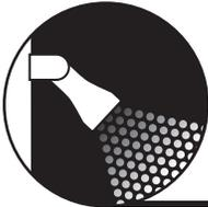
Downlighting is illuminating an object or surface from above. Downlighting can be used to highlight specific garden elements and functional areas. Also used for illuminating large spaces for safety, security or recreational purposes.
