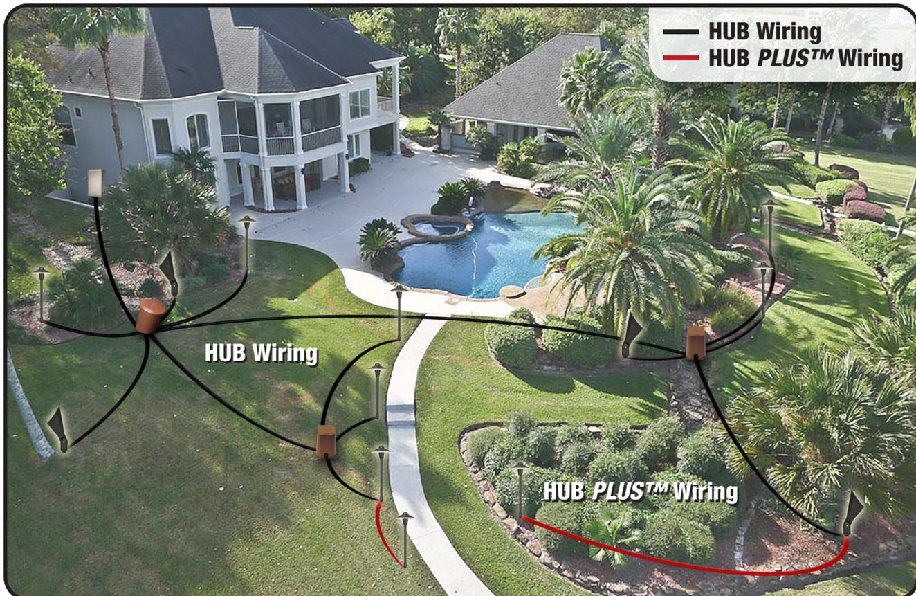
Flexibility is essential as landscapes continue to grow and change over time. The Elements™ Series features an auxiliary 1' wire lead, in addition to the 15' standard wire lead, on most fixtures. The new 1' FLEX™ Auxiliary Lead enables unmatched flexibility and makes future expansion easy as trees grow and the landscape develops.
